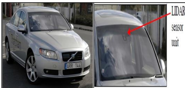
Fig.6: LIDAR Sensor Unit
