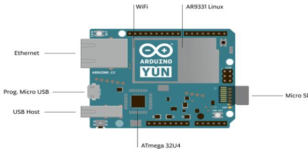
Fig.3 Arduino Yun microcontroller
