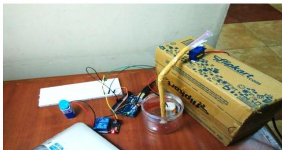
Fig.7 Setup of water spray system
