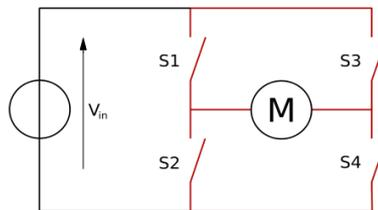
Fig.10 Structure of H-bridge
