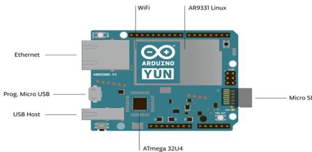
Fig.3 Arduino Yun microcontroller
