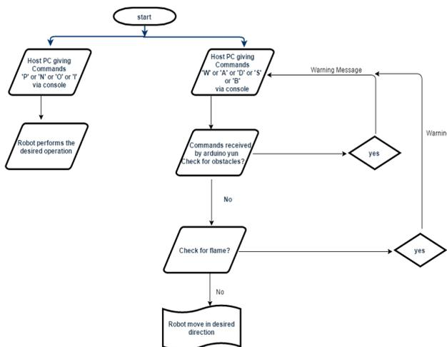
**Fig.16** Flowchart of operations performed by the robot
