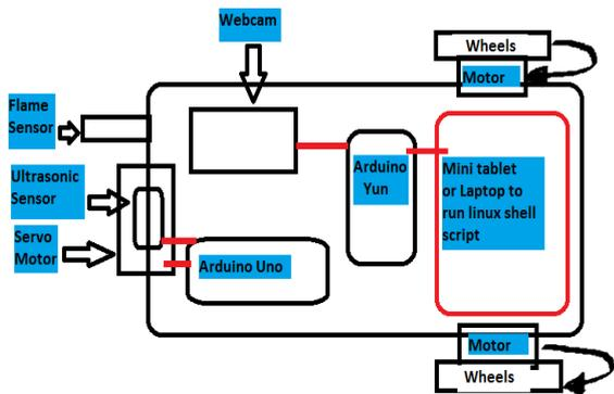
Fig.1 Components of designed robot (Top View)
