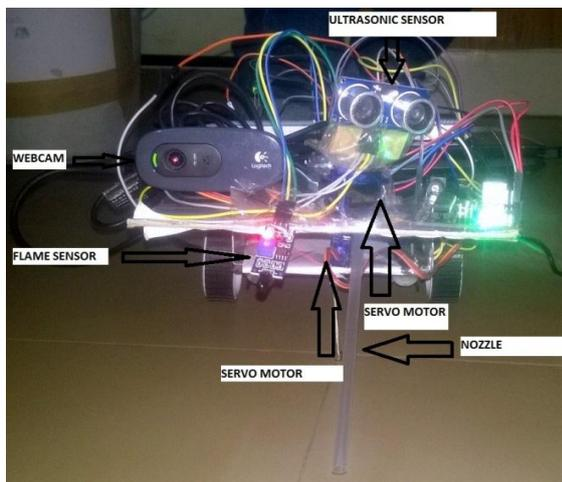
Fig.2 Design of fire extinguishing robot
