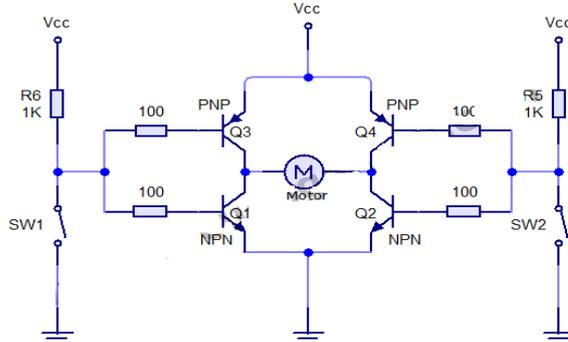
Fig.9 Circuit diagram of L293 H-bridge
