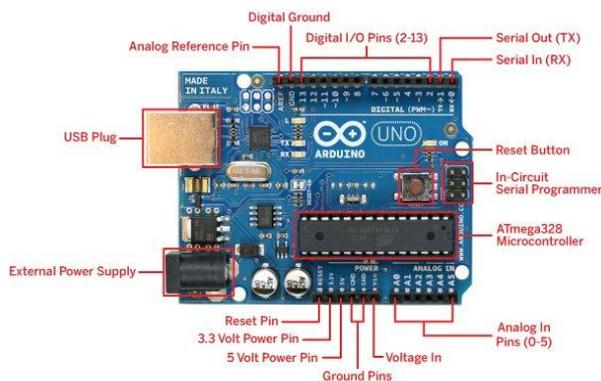
Fig.4 Arduino Uno microcontroller
