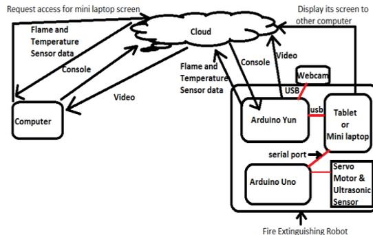
**Fig.11** Block diagram of the system
