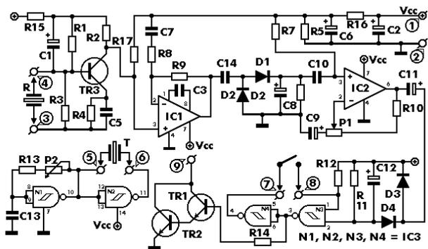
Fig.6 Circuit diagram of Ultrasonic sensor
