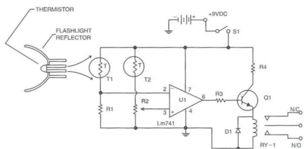
Fig.5 Circuit diagram of flame sensor
