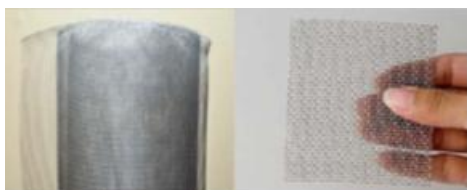
Fig.1: Screen mesh wick used in the heat pipe
