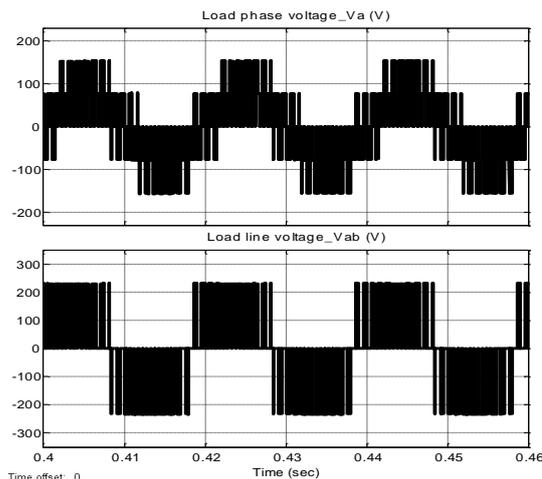
**Fig: 12** Phase and line voltage waveforms with modulation index of 0.9
