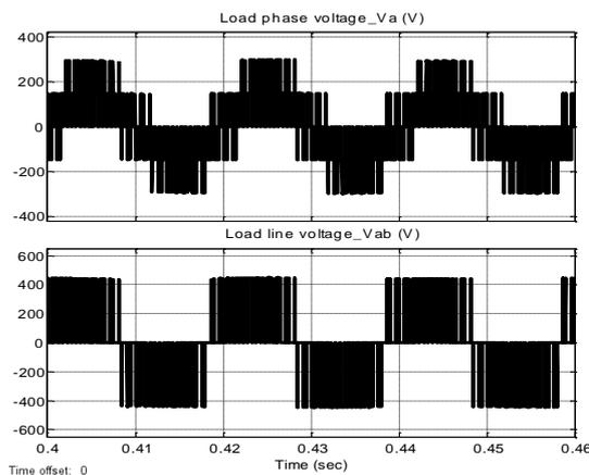
**Fig: 11** Phase and line voltage waveforms with modulation index of 0.8
