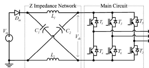
Fig: 1 Conventional Z-source inverter
