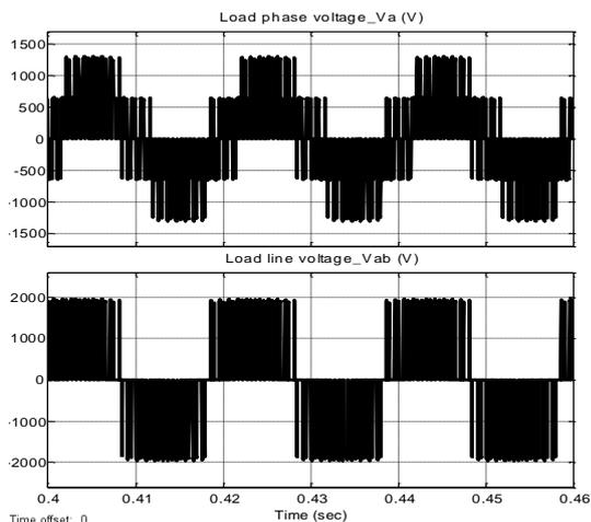
**Fig: 10** Phase and line voltage waveforms with modulation index of 0.7
