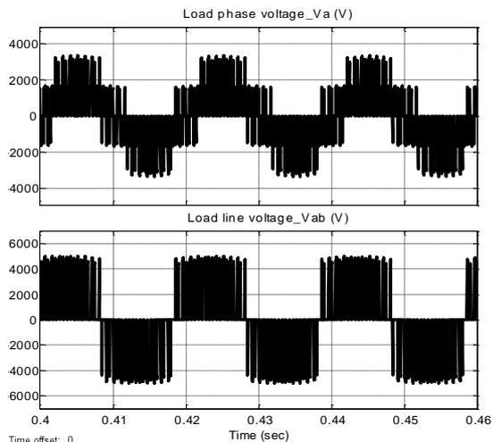
**Fig:9** Phase and line voltage waveforms with modulation index of 0.6
