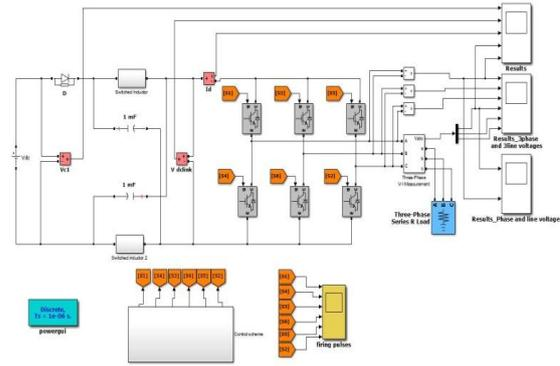
Fig: 6 Simulink model of Z-source inverter with switched inductor
