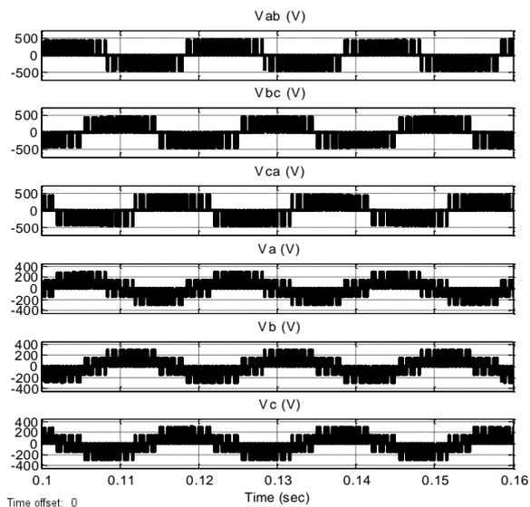
**Fig: 8** Scope results of ZSI-SI showing three phase load line and phase voltages
