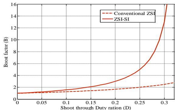
Fig. 4 Boost ability comparison of the classical Z-source impedance network and the Z-source impedance network with switched inductor
