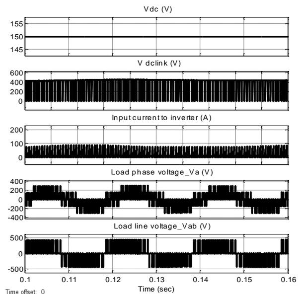
Fig: 7 Simulation results of ZSI-SI showing (a) input DC voltage, (b) DC link voltage after Z-network, (c) Input current to the inverter, (d) Load phase voltage, (e) Load line voltage
