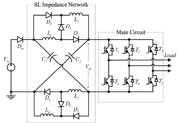
Fig. 2 Z-source inverter with switched inductor
