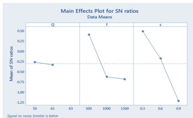
Fig.7: Main effects plot for S/N ratios of factor effects on surface roughness
