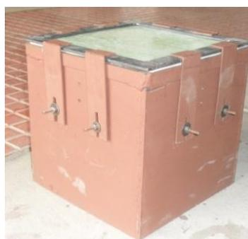
**Fig.5** Drop box setup
