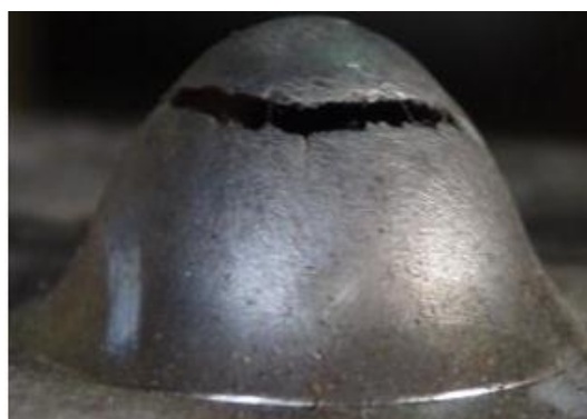
Fig. 5.b shows the crack in sheet (after fracture)
