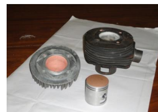
Plate 1 Photographic view of copper coated piston, liner and copper coated cylinder head
