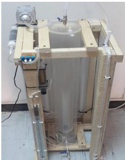
**Fig.2** Photographic view of the experimental airlift reactor in use
