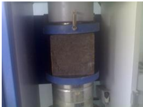
Fig. 6 Cubic in compression testing machine
