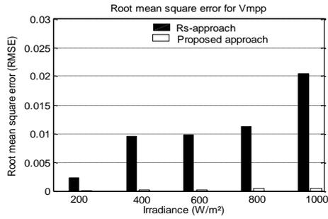
**Fig.10.** Root means square error for  $V_{mpp}$  for the proposed approach and the Rs-approach for MSX60 module for various irradiances
