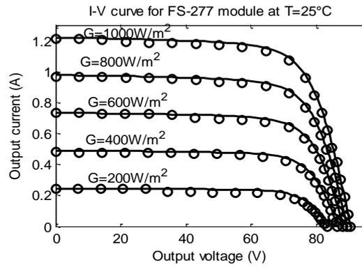
**Fig.14.** I-V curves of proposed approach and experimental values of the FS-277 module for various irradiances
