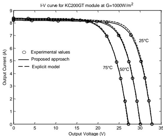
**Fig.3** Current-voltage curves of proposed approach and explicit model of the KC200GT module for various temperatures
