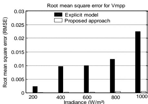
Fig.4. Root means square error for  $V_{mpp}$  for the proposed approach and the explicit model for KC200GT module for various irradiances
