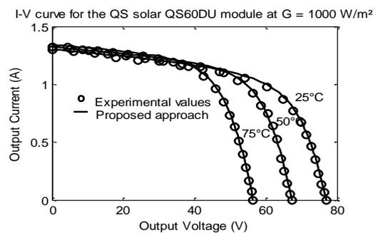
**Fig.17.** I-V curves of proposed approach and experimental values of the QS60DU module for temperatures
