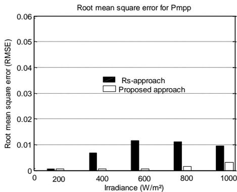
**Fig.12.** Root means square error for  $P_{mpp}$  for the proposed approach and the Rs-approach for MSX60 module for various irradiances
