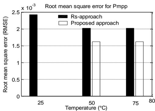
**Fig.13.** Root means square error for  $P_{mpp}$  for the proposed approach and the Rs-approach for MSX60 module for various temperatures
