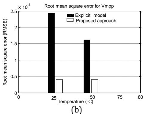
Fig.5. Root means square error for  $V_{mpp}$  for the proposed approach and the explicit model for KC200GT module for various temperatures
