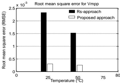
**Fig.11.** Root means square error for  $V_{mpp}$  for the proposed approach and the Rs-approach for MSX60 module for various temperatures
