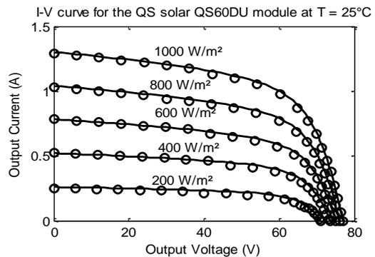
**Fig.16.** I-V curves of proposed approach and experimental values of the QS60DU module for irradiances
