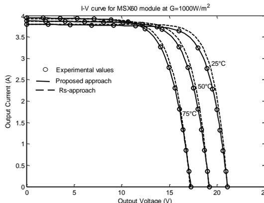
Fig.9. I-V curves of proposed approach and explicit model of the MSX60 module for various temperatures
