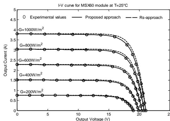
Fig.8. I-V curves of proposed approach and explicit model of the MSX60 module for various irradiances
