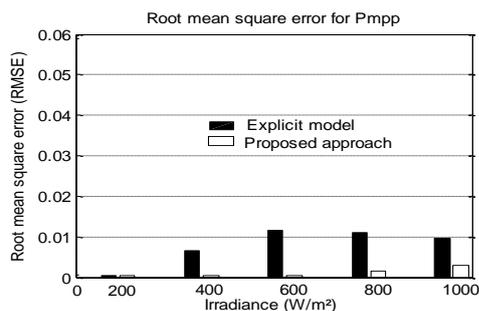
Fig.6. Root means square error for  $P_{mpp}$  for the proposed approach and the explicit model for KC200GT module for various irradiances
