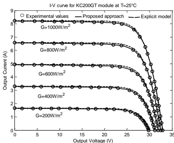
**Fig.2** Current-voltage curves of proposed approach and explicit model of the KC200GT module for various irradiances
