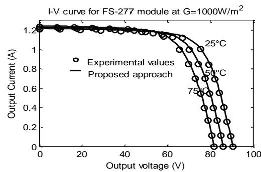
**Fig.15.** I-V curves of proposed approach and experimental values of the FS-277 module for various temperatures
