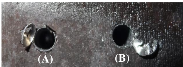
Fig 2. Burrs formed in D2 (A) Uniform Burr with cap (B) Uniform Burr with chips
