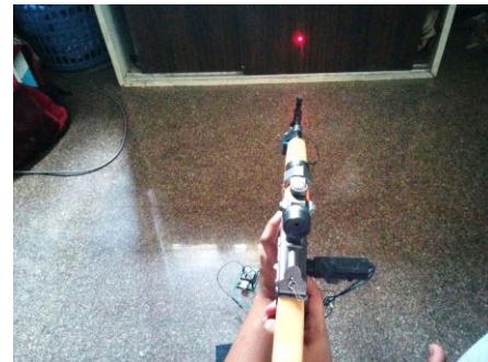
Fig 13: Laser mounted on the gun and poised along the line of fire
