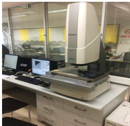
Fig.5 Nikon NEXIV VMR-3020 CNC Video measuring System
