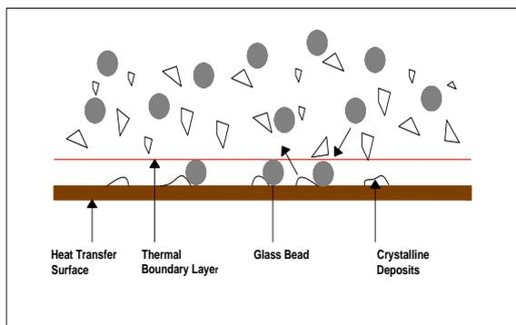
**Fig.7** Schematic diagram illustrates the cleaning action of glass beads and the breaking of thermal boundary layer (Kang et al., 2011)
