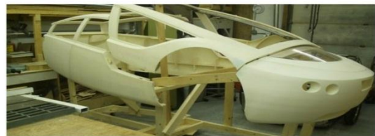
Figure shows the chassis model made using Fused Deposition Modeling technique
