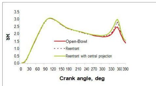
Fig.6 Swirl Ratio vs. Crank angle for different combustion chamber
