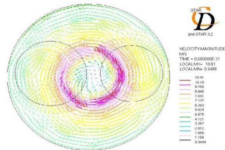
Fig.7 Velocity vector in the bowl entry at 360 deg CA ATDC Open bowl
