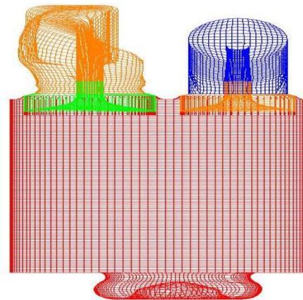
**Fig.3** Computational domain of reentrant with central projection combustion chamber geometry
