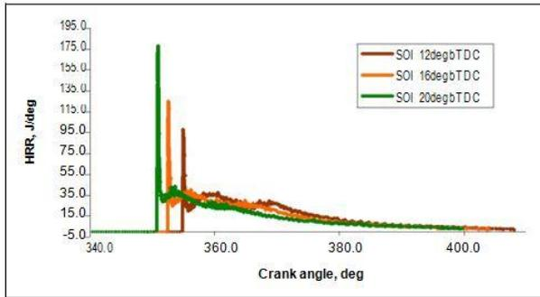
**Fig.16** Heat release rate for various injection timing
