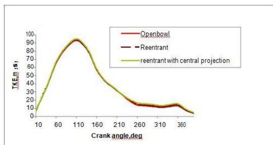
Fig.10 Mass averaged turbulent kinetic energy for different combustion chamber geometries.
