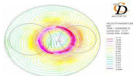
Fig.8 Velocity vector in the bowl entry at 360 deg CA ATDC - Reentrant
