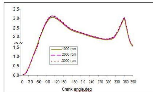
Fig.13 Mass average swirl ratio for different engine speed – reentrant with central projection combustion chamber
