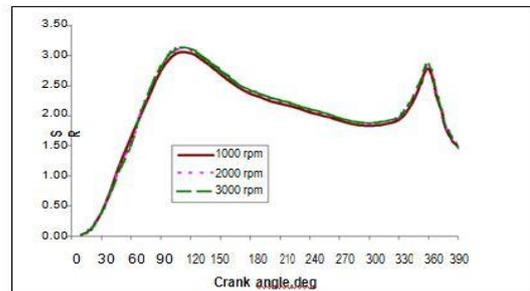
Fig.12 Mass average swirl ratio for different engine speed – reentrant combustion chamber
