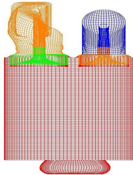
**Fig.2** Computational domain of reentrant combustion chamber geometry
