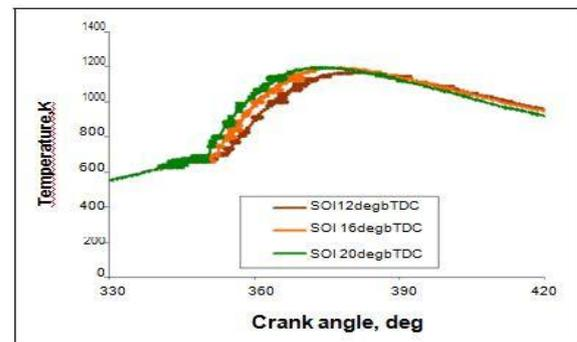
**Fig.15** Cylinder average temperature for various injection timing
