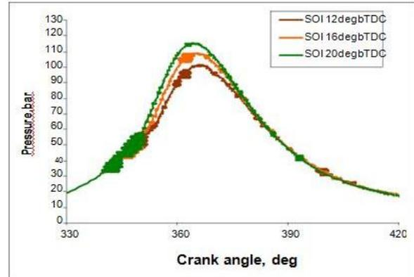
**Fig.14** Cylinder average pressure for various injection timing
