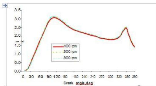
Fig.11 Mass average swirl ratio for different engine speed – open bowl combustion chamber
