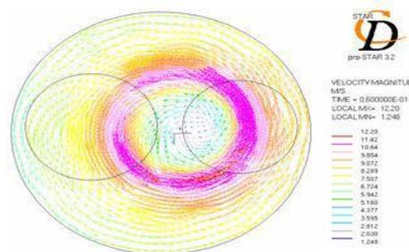
Fig.9 Velocity vector in the bowl entry at 360 deg CA ATDC -Reentrant with central projection.
