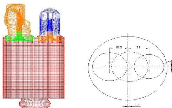
**Fig.1** Computational domain of open bowl combustion chamber geometry
