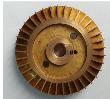
Fig.1 Pictorial view of the impeller having radial blades
