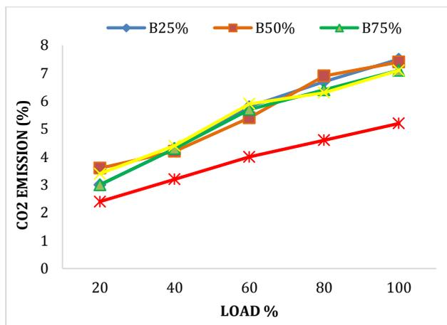
Fig 3 Variation of CO<sub>2</sub> emission with load for different blends
