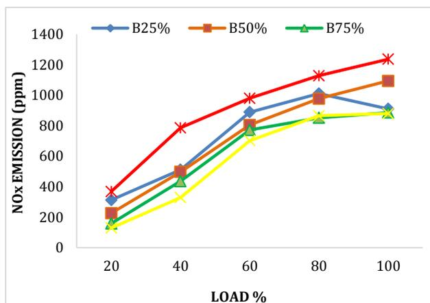
Fig 4 Variation of NO<sub>x</sub> emission with load for different blends
