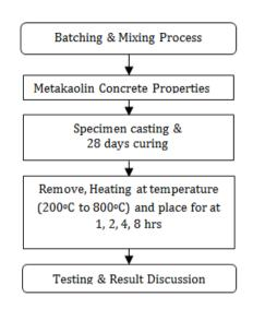
3.2 Test conducted on hardened concrete confirming to IS 516-1959
