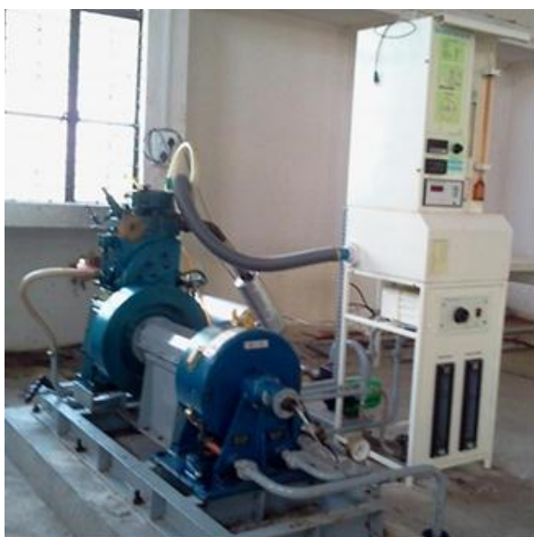
Fig.1 Photograph of VCR Engine Test Setup
