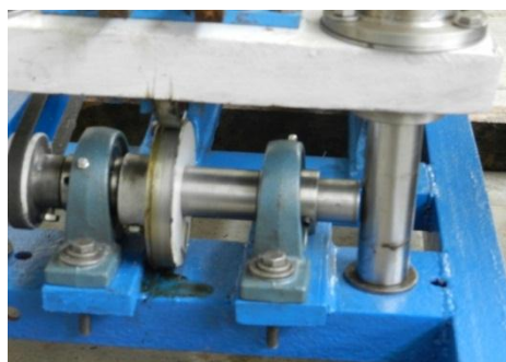
Fig Photograph of Previously used Cam and follower mechanism Sinusoidal motion given by Cam,
