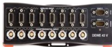
Fig DEWE 43 V Data acquisition system
