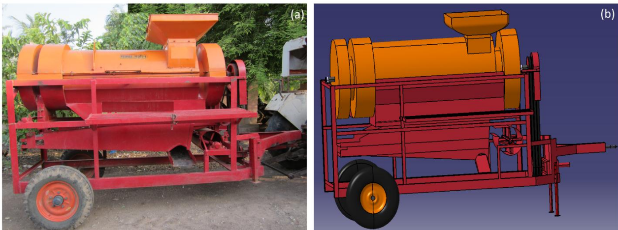
Fig. 1 Maize sheller cum dehusker (a) Actual machine (b) 3D model
