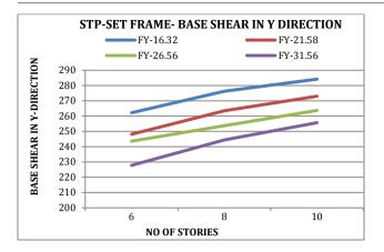
There is rise in base shear value with respect to the increase in the storey height. It's clearly seen that the increase in base shear in x direction is more from 6 stories to 8 stories than the 8 story to 10 story. But in case of Base shear in y direction the rate of increase is almost the same. We can see the effect of no bays influencing the base shear value.
