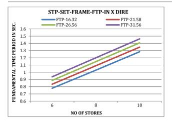
The linear rise in fundamental time period is seen with respect to the rise in number of stories. Also here we can see the difference in time period values in both types of frames. As earlier comparisons, here also, the vales of the fundamental time period are seen less than that of the step back frames.
