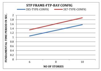
For a given number of bay, the time period increases with increase in number of storey. For a given number of storey, the time period increases with increase in number of bay. The time period increases mildly with increase in number of bay. The nature of variation observed is nonlinear for all number of bays.
