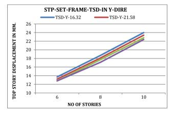
The rate of increase in top story displacement is proportional to the height of the building or in other word, the no of stories in consideration. The slop angle influences the displacement values. It can be seen that the 26.56 degrees and 31.56 degrees at the 6 story height does not make significant difference but as the story height increases the values are clearly distinct.
