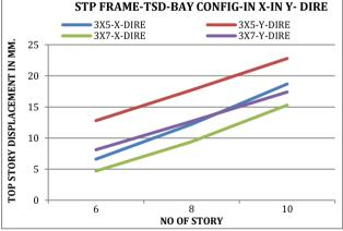
The top story displacement values are seen variant for the bay values as the no of bay increases the displacement changes. This change can be encountered as, as the difference between the number of bays in x and y direction increases the displacement seen increased when the rest of the parameters are same. Also the number of stories increases the top story displacement increases.
