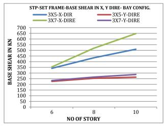
As the number of stories increases with the increase in the number of bays, significant rise is seen in the base shear value. The rate of increase is non-linear in nature. The base shear in y direction for both type of frames seen similar at the less number of stories, but after the story 8 values it seems distinct.
