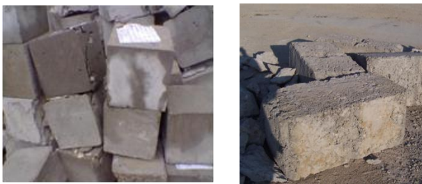
Figure 1 Concrete specimen (left) and concrete blocks (right) used for the production of aggregates inhomogeneous and homogeneous origin, respectively.
