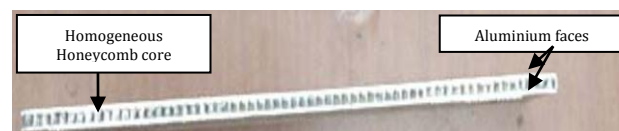
Fig.2. Sandwich beam configuration Al/Honeycomb/Al
