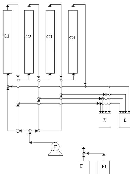
**Fig. 1** The SMB system used for fructose separation, where C1, C2, C3 and C4 are the experimental columns measuring 1 m in length and 25 mm in inside diameter, F is the Feed (date syrup), El is the Eluent (distilled water), E is the extract (liquid with the separated fructose), R is the Raffinate (liquid with residual sugars such as glucose), and P is the pump.
