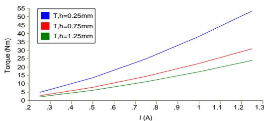
Fig. 5 Torque vs. Current for configuration 1 without saturation
