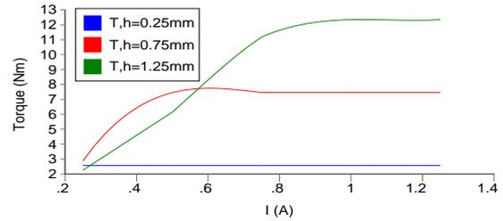
Fig. 6 Torque vs. Current for configuration 1 with saturation
