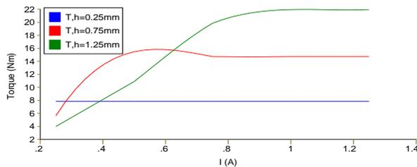
**Fig.8** Torque vs. Current for configuration 3 with saturation
