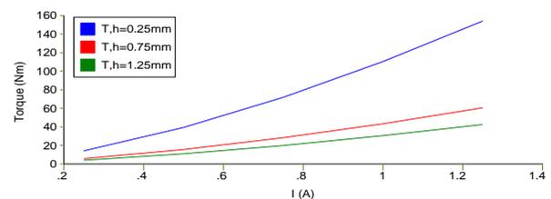
Fig. 7 Torque vs. Current for configuration 3 without saturation
