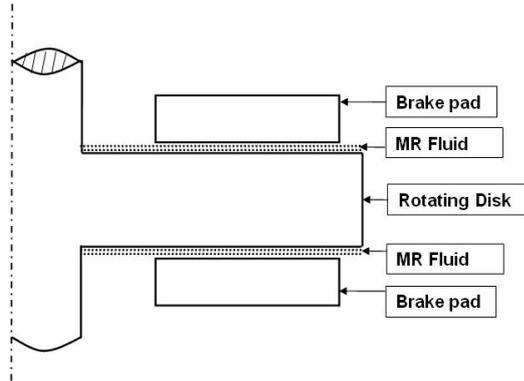
Fig.1 Block diagram of MR Brake
