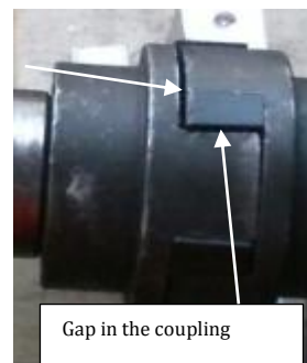
Fig. 13 Gap between the jaw of the coupling due to permanent deformation of rubber
