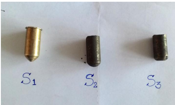
Fig. 2.7 Final finished specimen of size 10mm× 30mm
