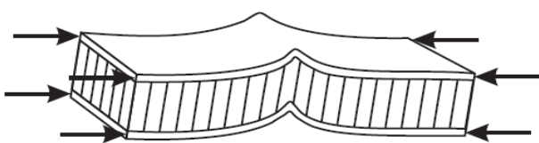
Fig 4.3 Panel Buckling of honeycomb plate
