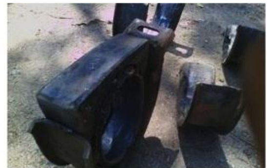
Fig.9 crack at the fillet region in working condition
