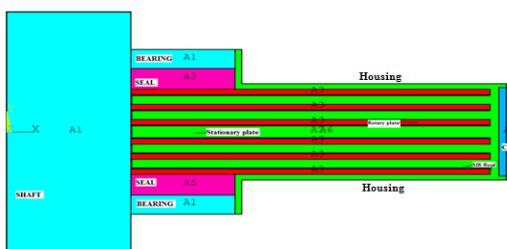
Fig.10 Modified MR Brake assembly
