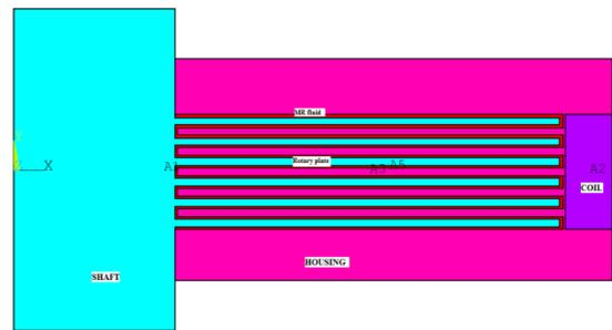
Fig.6 Simple 2D Axisymmetric Model of MR Brake
