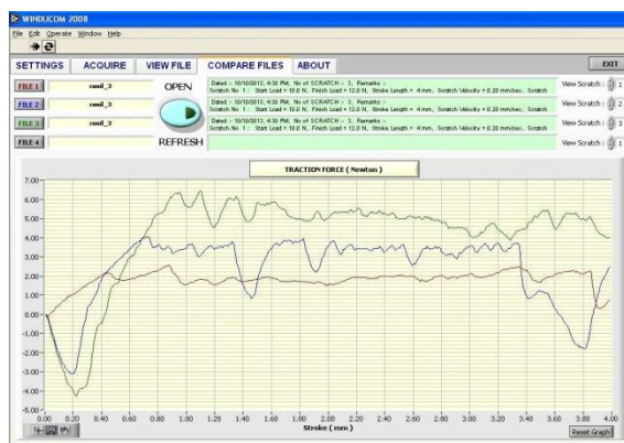
Figure 3: Comparison between Traction force and Stroke for scratch 3 of Ni-Al 2 O 3 coated specimen
