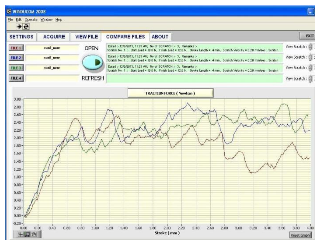
Figure 2: Comparison between Traction force and stroke for three scratches of Ni-TiO 2 Al 2 O 3 Coated specimen
