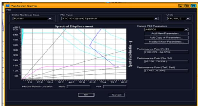
Figure 2.6 Capacity Spectrum Curve
