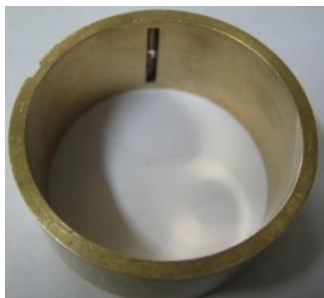
Figure 3 Bearing with only axial groove
