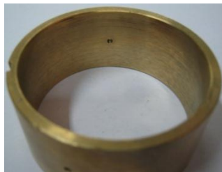
Figure 2 Bearing without groove
