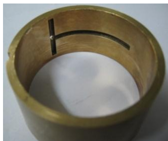
Figure 5 Bearing with combined axial and circumferential groove
