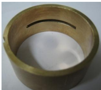
Figure 4 Bearing with only circumferential groove
