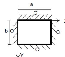
**Figure 4** Boundary conditions of Levy-type plate
