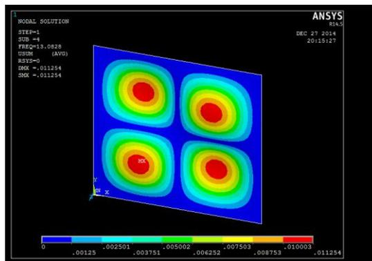
**Figure 10** First Four modes for the 10x10m CCCC isotropic plate
