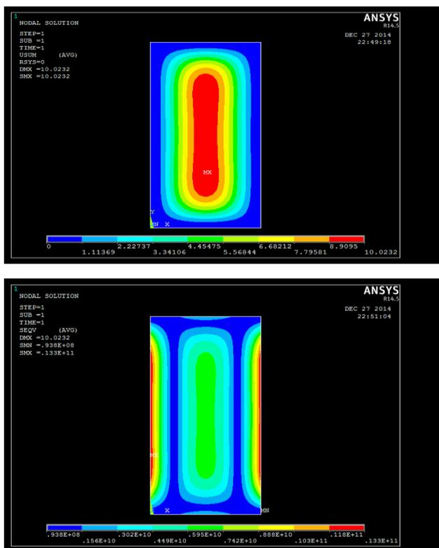
**Figure 9** Max stress, deflection due to uniform loading for CCCC  $1 \times 2 \text{m}$  orthotropic Plate
