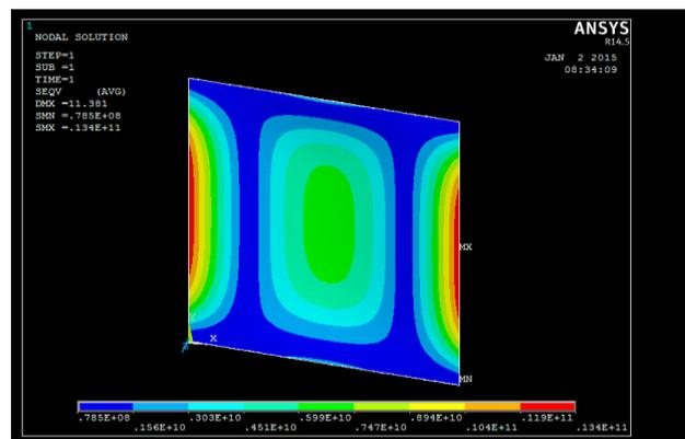
Figure 8 Max stress, deflection due to uniform loading for CCCC 1x1.2m M1 orthotropic
