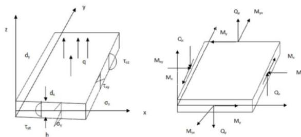
Figure 1 Out of plane stresses
