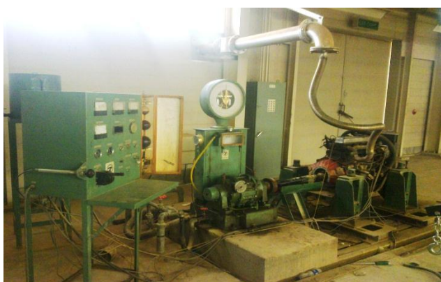
Fig.1 The engine coupling with dynameters used in this experimental
