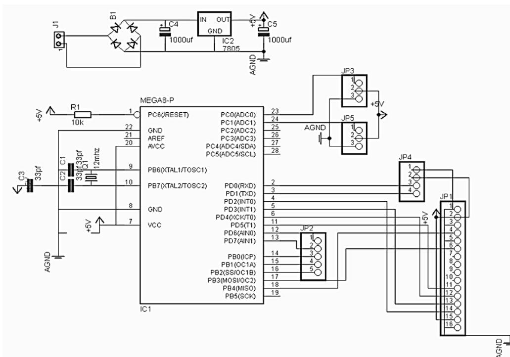
Figure 2 Schematics circuit diagram of wireless sensor network
