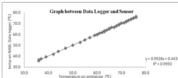
**Figure 4** Graph plotted between the temperature range of the NABL Data logger and the Thermocouple sensor
