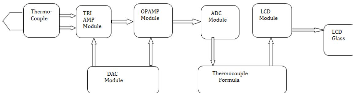
Figure 1 Block diagram of the wireless temperature monitoring system
