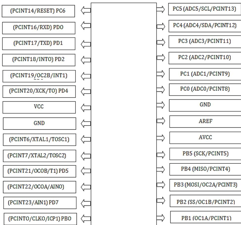
Figure 3 Show the pin configuration of AVR Atmega328
