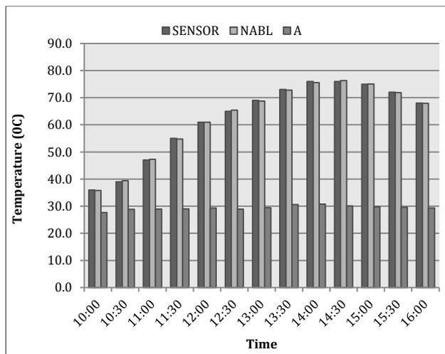
**Figure 6** Variation on temperature taken by the Temperature sensor, NABL lab sensor and the ambient temperature with different time interval
