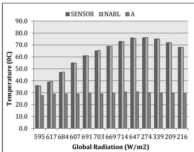
**Figure 7** Variation on temperature taken by the temperature sensor, NABL lab sensor and the ambient temperature with different Global radiation (W/m<sup>2</sup>)
