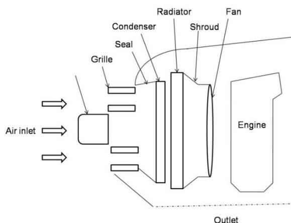
Fig.1 Front End Flow
