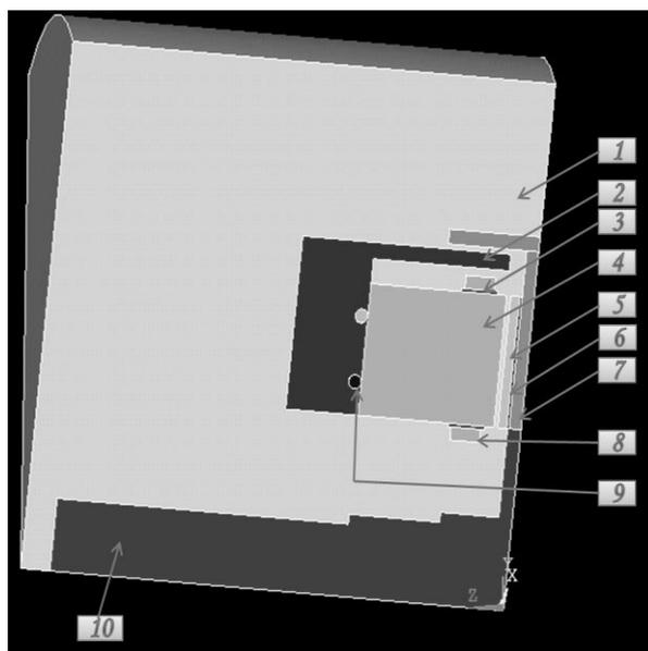
Fig.4 The 3D model of 1/16 of the AFIR (1 air, 2 casing, 3 Pressboard, 4 stator, 5 PM, 6 glue, 7 rotor, 8 copper windings, 9 cooling pipes, 10 shaft)
