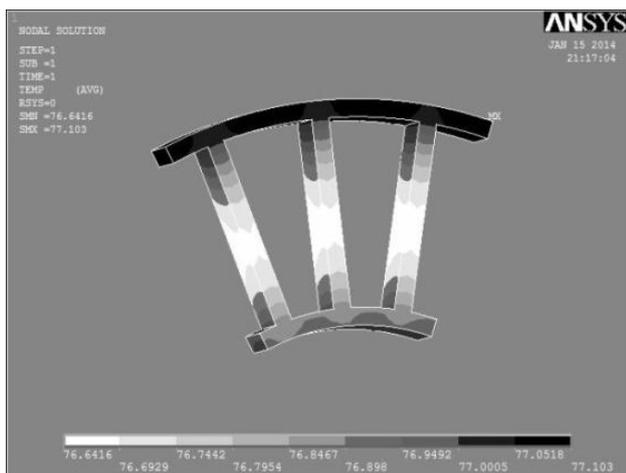
Fig.5 Temperature distribution through the windings
