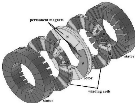
Fig.2 Electromagnetic machine with a disc rotor built by Tesla
