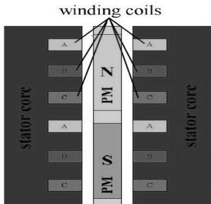
Fig.3 2D side view of slotted stator AFIR
