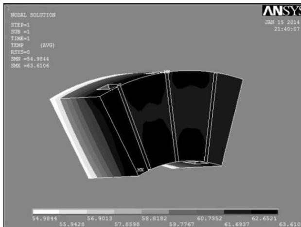
Fig.6 Temperature distribution through the stator yoke
