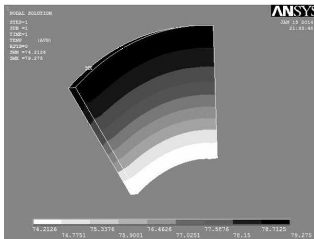
Fig.7 Temperature distribution through the PM
