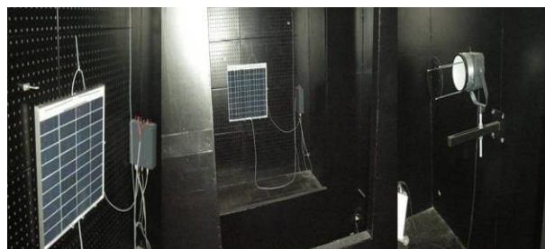
Fig.3 Quick sun 700A sun simulator for I~V measurement
