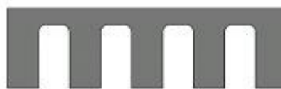
Fig 5: Rectangular micro channel with corner radius
