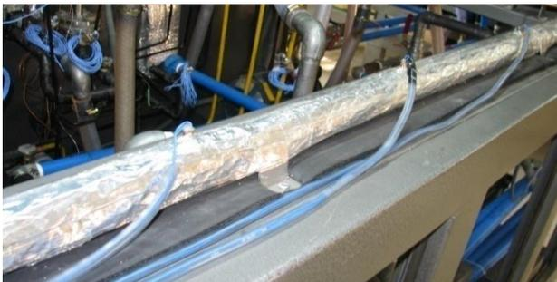
**Fig.3** Test Section of Insulated Horizontal Pipe
