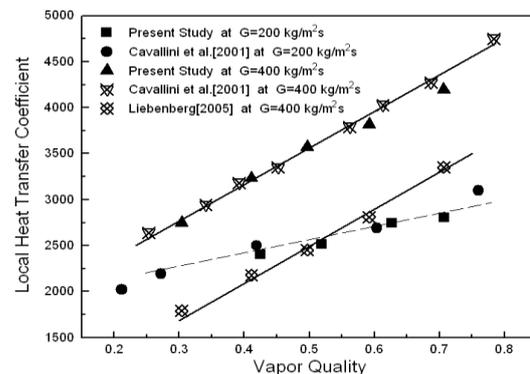
**Fig.4** Comparison of Local Heat Transfer Coefficient of Present Study with other Experimental Data from Literature
