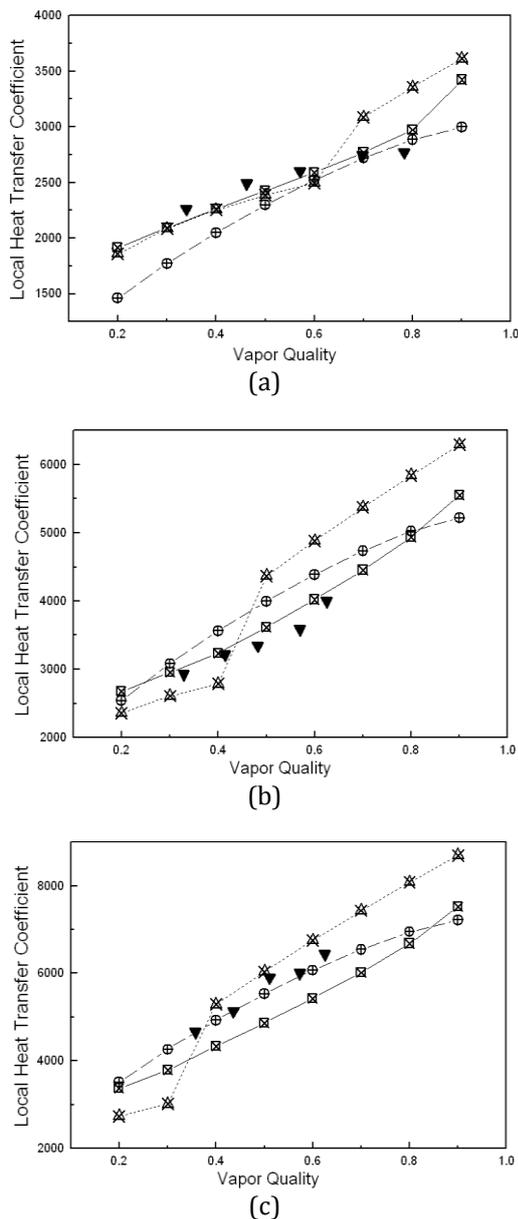
Fig.7 Comparison of Experimental Heat Transfer Coefficient of R134a with Correlations
