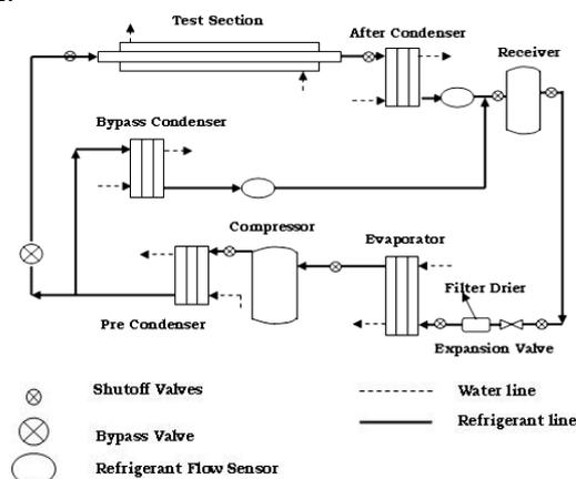
Fig.2 Schematic of Refrigerant Loop
