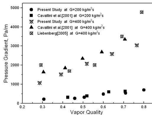
Fig.6 Comparison of Local Pressure Gradient of Present Study with Experimental Data from Literature
