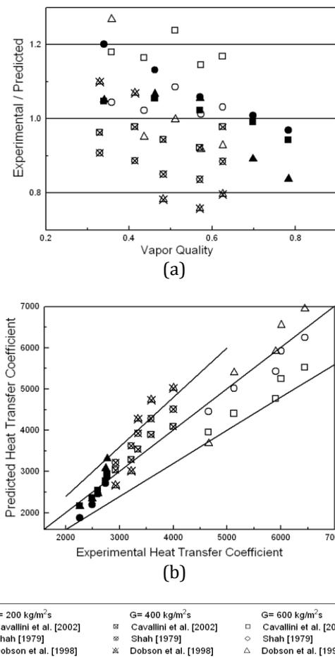
Fig.8 a) Deviation Graph b) Parity Graph for R134a
