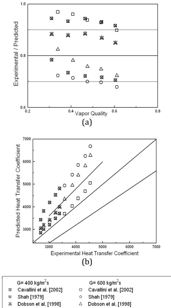
Fig.9 Comparison of Experimental Heat Transfer Coefficient of R407C with Correlations
