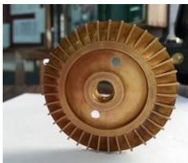
**Fig. 2** Pictorial view of the pump impeller
