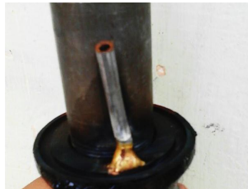
Fig. 4: Inside view of Bottle jack (Model no. – QYLS5) after welding the pipe
