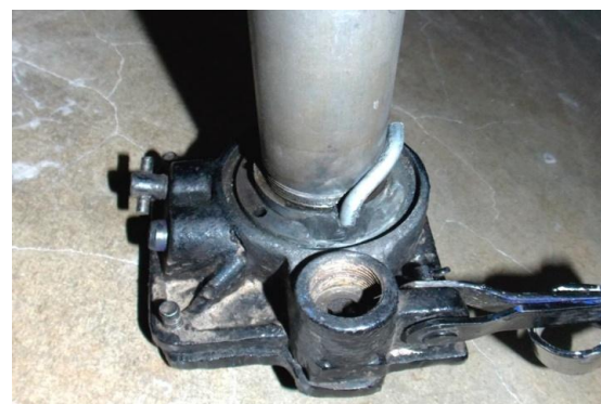
Fig. 5: Inside view of Bottle jack (Model no. – QYLS5) after using the adhesive and bending the pipe
