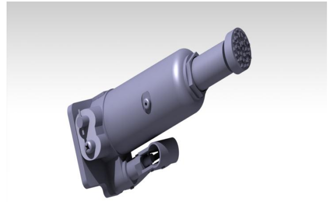
Fig. 7: 3-D drawing of the bottle jack – Model No. QYLS5 after adopted changes
