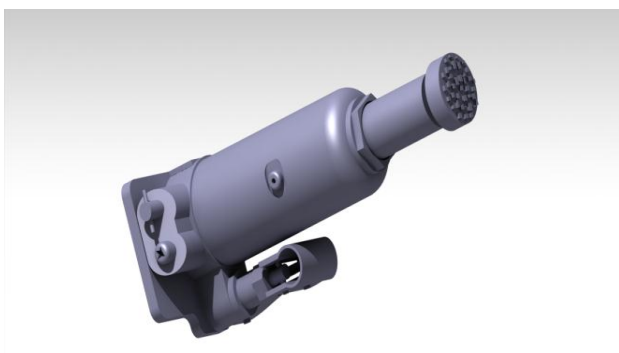
Fig. 2: 3-D drawing of the bottle jack – Model No. QYLS5 before adopted changes
