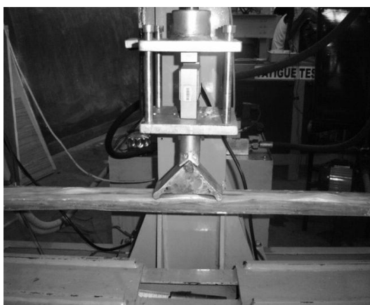
Fig. 3 Static load test
