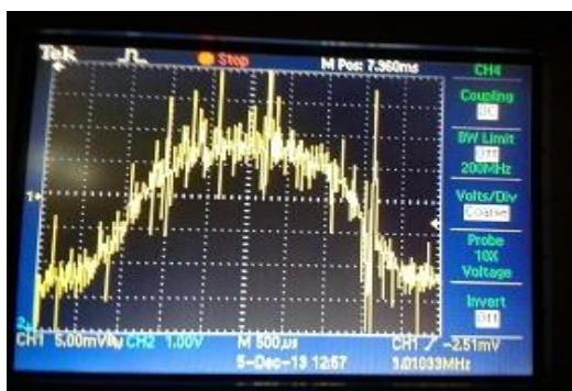
Fig.10: The photoresponse time of fabricated SnO 2 UV detector. The time base on x-axis is 500 \mu s/div
