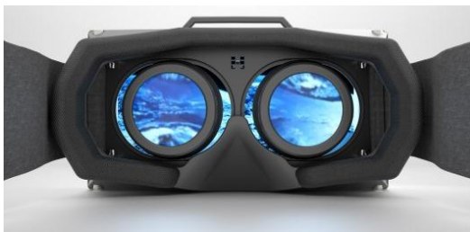
Fig. 3 The Rift with its immersion-producing lenses
