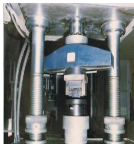
Fig.3 Daratec machine for compression test
